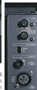
NX-5A Rear Panel Bi-amplifier with controls for overall output level control, tweeter level control (±3dB) cut/boost, and selectable +2dB / 0dB / -2dB LO EQ control at around 55Hz.
