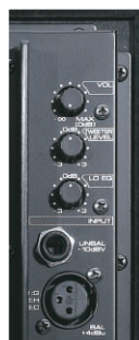
NX-6A Rear Panel Bi-amplifier with controls for overall output level control, tweeter level control (±3dB) cut/boost, and variable LO EQ control: with ±3dB of cut/boost at around 55Hz.
