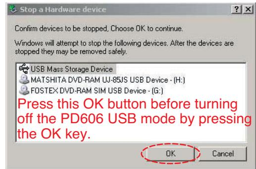
Press this OK button before turning off the PD606 USB mode by pressing the OK key.
