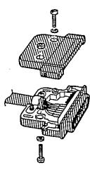
Remove the connector shell and exchange pin assignments between:
