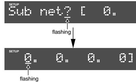
2. Use the shuttle to move the flashing digit and use the JOG dial to select a value.
