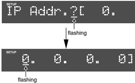
2. Use the shuttle to select the flashing digit and use the JOG dial to select the value.
