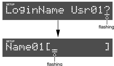
2. Use the shuttle to move the flashing digit and use the JOG dial to select a character.
