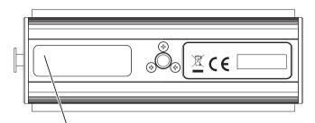
AR501 has a pit on the bottom chassis to stick a user label for the users' convenience. Use it for attaching a label in the way you like such as company ID and administrative control number plate. Since the pit is retracted, it avoids the label getting damaged when attaching a tripod.
