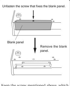
Keep the screw mentioned above, which will be used in step 4 below after installing the CD-RW drive. 2 Turn the VF160 over and insert the CD-1A into the slot on the front panel.
