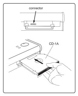
Use two screws supplied with the CD-1A to fix the CD-1A to the VF160 from the front panel. Tighten the screws with a screwdriver.
