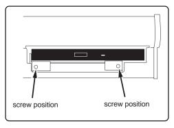
Use the screw you removed in step 1 to fix the blank panel supplied with the CD-1A to the front panel.
