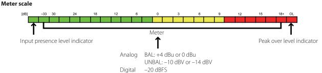
The meter scale has 26 dot LED consisting of a 24 dot level meter, an input presence level indicator and a peak over level indicator. You can choose from four combinations of PEAK and VU to be displayed on the meter ("DIP switch settings" ( $\Rightarrow$  page 4)).
