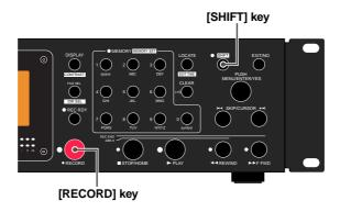
**<Note>:** Pressing the [RECORD] key while the SHIFT mode is active during recording turns off the shift mode. To divide the track again, do not forget to press the [SHIFT] key to turn on the shift mode before pressing the [RECORD] key.
