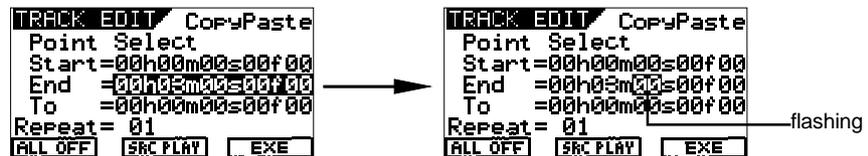
For example, if you can shift the end point 5 seconds backwards, change the current data ("00h 03m 00s 00f 00") to "00h 03m 05s 00f 00" by using the [JOG] dial to set the second digit to "05".
